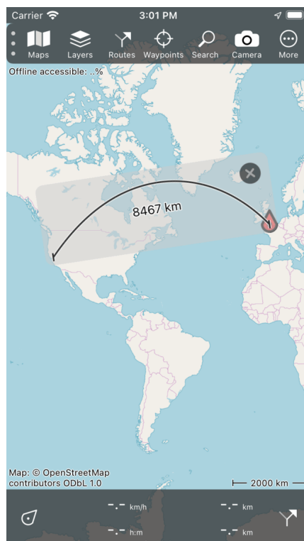
Fig. 3: The curve on the map ruler is not a straight line but a geodesic.
