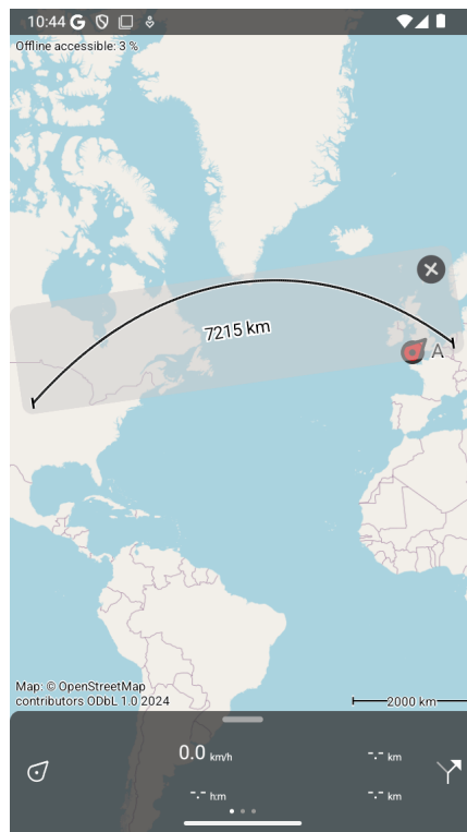
Fig. 3: The curve on the map ruler is not a straight line but a geodesic.
