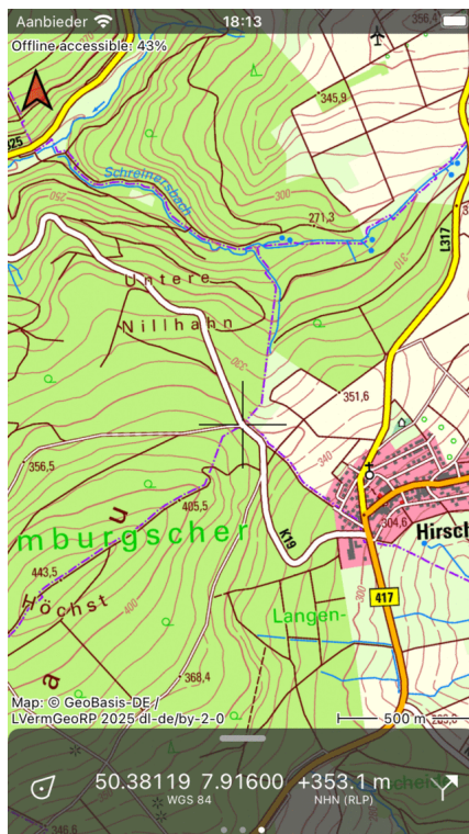
Fig. 1: The terrain height is shown next to the coordinates on the dashboard.
